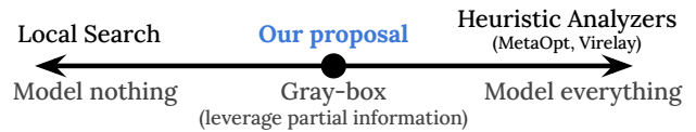
FIGURE 1: We propose a gray-box approach that uses gradient to analyze performance of learning-enabled systems. Existing white-box heuristic analyzers have limited expressiveness and scalability [13, 32, 33] as they require an exact model of the system (including the DNN) in optimization or logic. Local search methods fail to find bad inputs as they ignore all the details about the underlying system.
